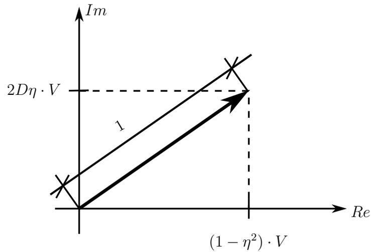
$$\begin{aligned} \Rightarrow 4D^2\eta^2V^2 + (1 - \eta^2)^2V^2 &= 1 \\ \Rightarrow V &= \frac{1}{\sqrt{(1 - \eta^2)^2 + (2D\eta)^2}} = V_3 \quad (\text{Krafterregung}) \end{aligned}$$
